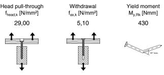
To obtain characteristic head pull-through capacity multiply parameter by outside crown width b and nominal diameter d
